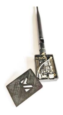
Figure 14 shows the development board inside a 3D printed prototype casing. These prototypes were used during the testing of the implementation.
