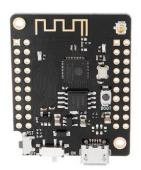
The Wemos TTGO ESP32 Mini was chosen as the development board. This is a very small PCB (printed circuit board) with a PCB antenna Figure 11 - Wemos and connector for an external antenna. The external antenna can be used to improve the connectivity between the Wi-Fi access points and Bluetooth scanning.
